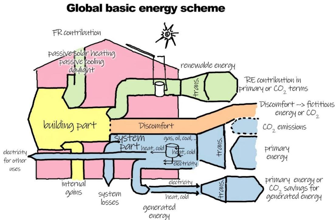
**Figure 8: Potential E-DYCE Free-running integration scheme**
