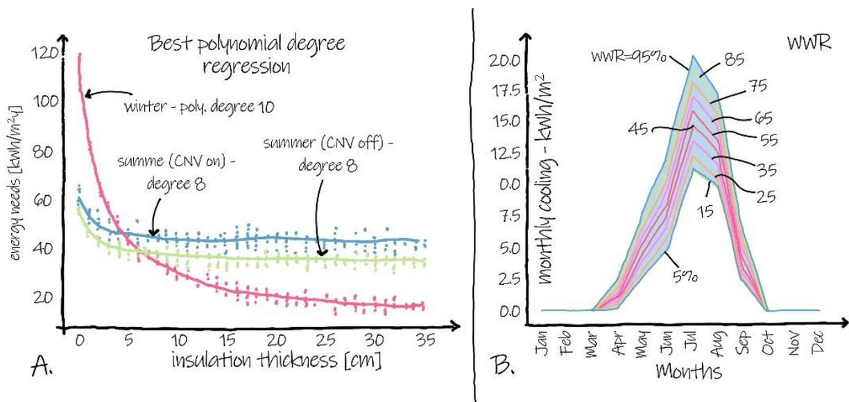
**Figure 23 – (a) Energy needs for space heating and cooling as a function of different envelope U-values to optimise insulation thickness, including random Gaussian occupancy values; (b) Monthly cooling energy needs as a function of different window-to-wall ratio. The two samples refer to different buildings and locations.**
