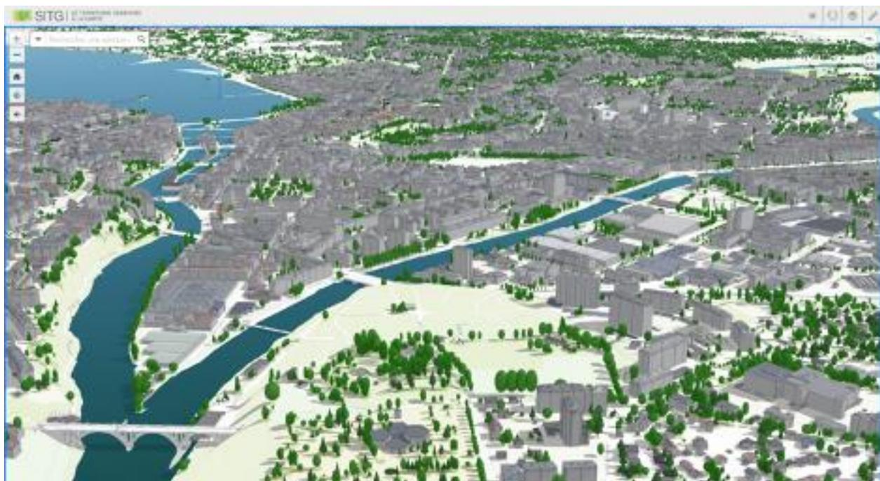
**Figure 6: Geneva canton 3D cadastre gives surface areas of facades, roofs, or heated reference areas.**
