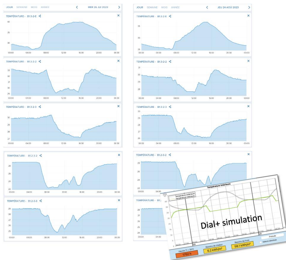
Figure 134 interior temperature in 6 offices during typical summer days in Cyprus (26 July and 24 Aug 2023)
